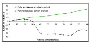
Fig. 3. The performance of Mandelbrot can be increased by forcing uniformity for more branches. However, if software overhead is added to ensure branch uniformity, increasing the number of affected branches increases overhead and can even result in degraded performance.
