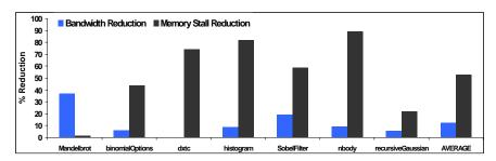
Fig. 17. Data herding improves performance by reducing memory stalls and bandwidth usage due to divergent memory requests.
