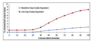
Fig. 4. While eliminating control divergence can increase performance, blindly forcing branch uniformity can result in degraded output quality.
