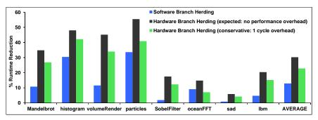
Fig. 12. Potential performance improvement for software and hardware branch herding. Although we don't expect any additional performance overhead for our implementation of hardware branch herding, we also show a conservative performance measurement assuming a 1 cycle overhead. Overhead is at most 1 cycle, since the additional logic (majority) is simpler than population count logic, which evaluates within a single cycle.
