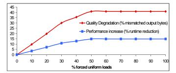
Fig. 6. Eliminating memory divergence (forcing more uniform loads) increases performance but also degrades output quality.
